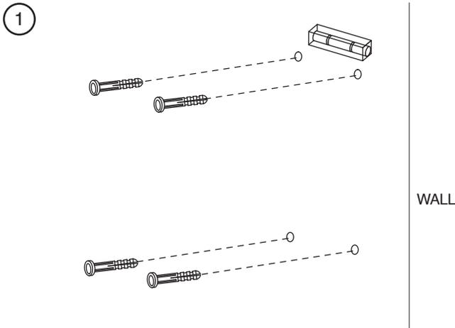
Determine the location for the wall sconce. Using a **level**, position **wall sconce assembly** and mark 4 hole positions on the wall. Set wall sconce assembly aside. Drill a pilot hole in the wall stud. If the wall stud is not available, drill a hole in the wall that is slightly smaller in diameter than the anchor. Insert 4 **plastic anchors** into holes. Gently tap **plastic anchors** into the wall until the flange of the anchor is flush.
