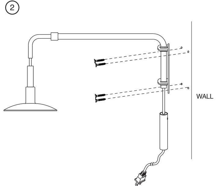
Align holes of **wall sconce assembly** with corresponding anchors in wall. Insert 4 **screws** through **wall sconce assembly** and into each **plastic anchor** as shown. Secure each screw with a **phillips head screwdriver**.
