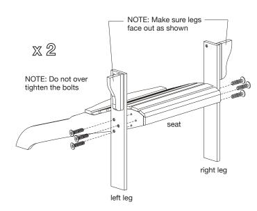
1) With the assistance of another adult, attached **left and right legs** to **seat** with 3 **small bolts** per side as shown. Secure, but do not over tighten, bolts using an **allen** wrench.
