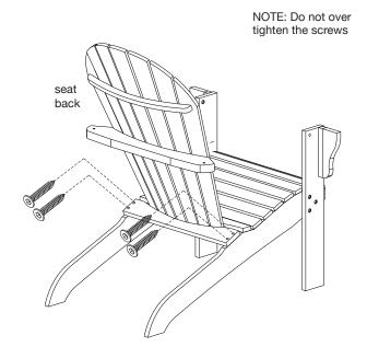
2) With the assistance of another adult, attached **seat back** to assembled unit with 4 **screws**. Secure, but do not over tighten, screws using an **allen wrench**.
