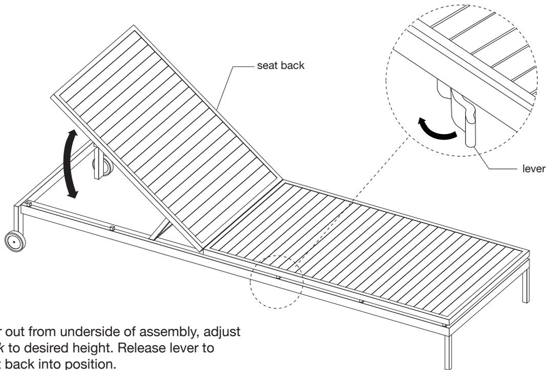
Pull *lever* out from underside of assembly, adjust *seat back* to desired height. Release lever to lock seat back into position.
