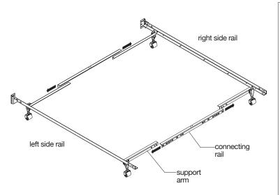
(3) Fit *pegs* of support arms of **right and left side rails** into corresponding *slots* of **connecting rails**. Refer to illustration. Firmly pull support arms and connecting rails apart until each peg securely engages each slot.
