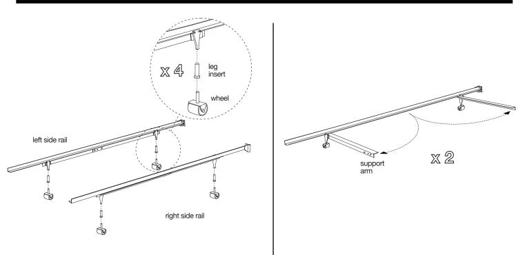
(1) With the assistance of another adult, fit **leg insert** and **wheel** into corresponding leg of **left and right side rails** as shown. Push down on each leg assembly to secure. (2) Unfold support arms of **left and right side rails**.
