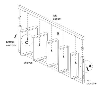
(3) A) Fit dowels of **crossbars** into **left upright**. Secure each crossbar with 1 **large bolt** as shown, using a **phillips head screwdriver**.
